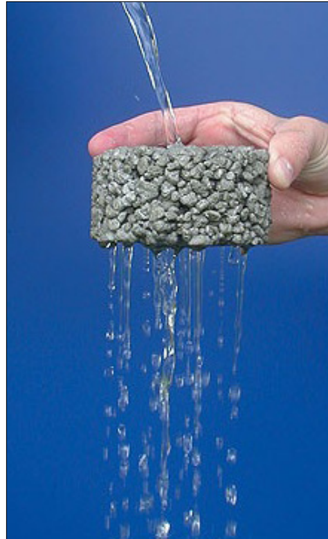
Figure 16: Pervious concrete allows water to flow through it into the ground below
